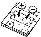
5) Install the new batteries, making sure the polarity (+ and -) is correct, and replace the battery compartment cover. (Make sure to replace the battery compartment cover--the batteries are not connected unless the battery compartment cover is in place.) Replace the back of the calculator by first hooking the 3 tabs on the top and then lowering the edge closest to you so you can replace the 2 screws.
