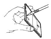
1) Install the Software Cartridge in the calculator. With a pencil or straightened paper clip and the calculator ON, push the "ALL RESET" button on the left side of the back of the calculator. You should see 4 stars in the display (2 on the left, 2 on the right). (On some calculators, there may be a white label over the "ALL RESET" button. If so, gently lift up the lower left corner to reveal it)
