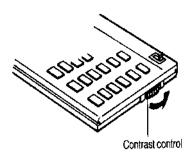
The calculator is equipped with a control to adjust the contrast of the LCD (liquid crystal display). While looking at the display from a position about 70 degrees above the keyboard, first increase the contrast until black squares are clearly visible behind the characters and then decrease the contrast slowly until the squares just disappear.
